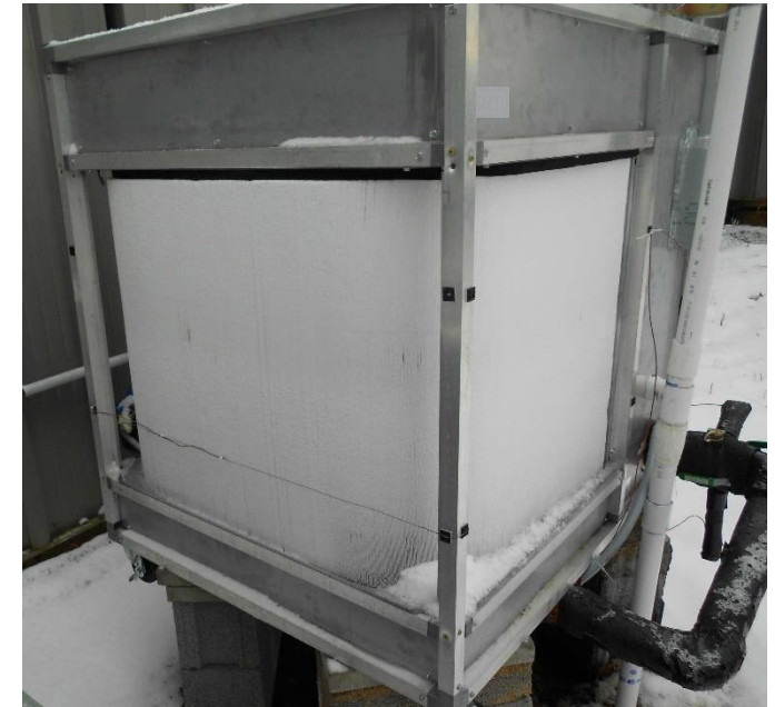
Experimenting with Defrost Control at Field Site
